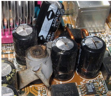
Figure 5: Capacitor damage due to overvoltage
